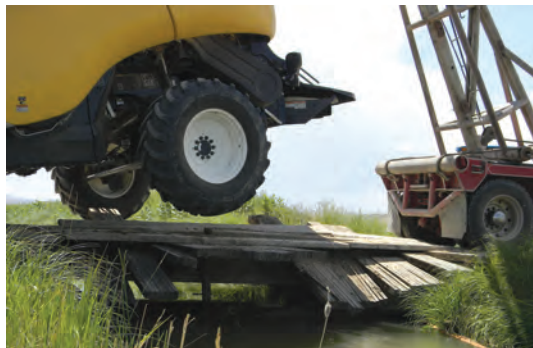
The crane operators lifted up the combine until the front drive tires were on solid ground. Dad then drove the combine forward as the crane operator kept the rear of the combine off the bridge.
