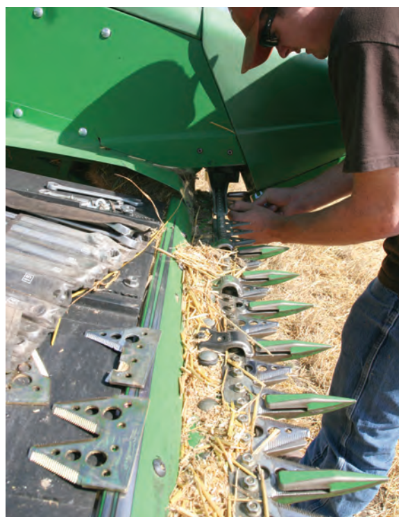
Leon fixes a broken knife on his header.
