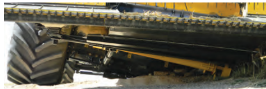
One of the header cylinders held much of the weight of the combine and was bent badly when the bridge broke.
