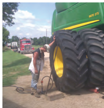
Dalton waits on more bolts to fasten on the outside dual.
