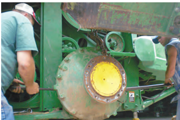
The men pry the boll gear loose from the machine.
