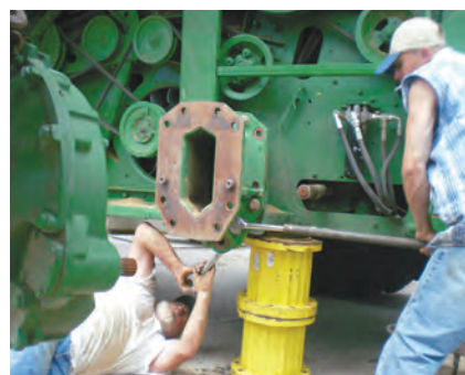
The guys tighten the bolts on the extension before putting the final torque on them.
