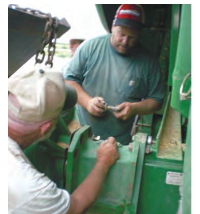
The boll gear is placed back on the extension and fastened.
