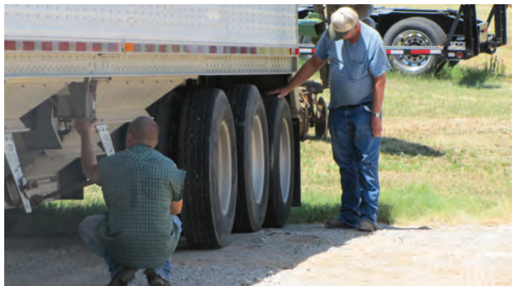
Jesse and Justin check to make sure the grain trailer's third axle lift valve is working properly.
